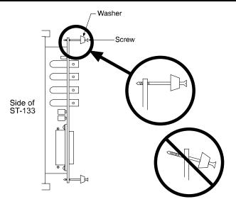
Figure 31. Module Installation
